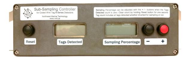
Clear the counter before changing the sampling percentage. If the buttons are pressed when the counter does not read zero, the right-hand display changes to the error message "Clear". Clear the counter and then resume changing the percentage.
