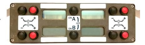
The left displays of each pair count fish exiting through the left door of the gate. The right-hand display of each pair counts exits from the right door. If your fish are exiting to the side opposite of the display, switch the probes in the gate doors.
