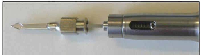
8. Screw the hub of the needle into the injector
