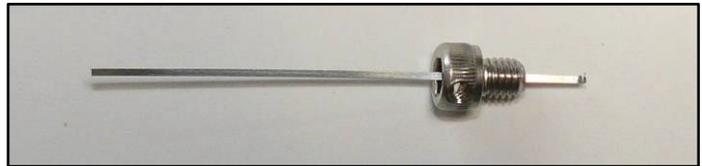
2. Insert the end screw into the threaded end of the plunger and tighten it. Check to see that the shim rotates freely.
