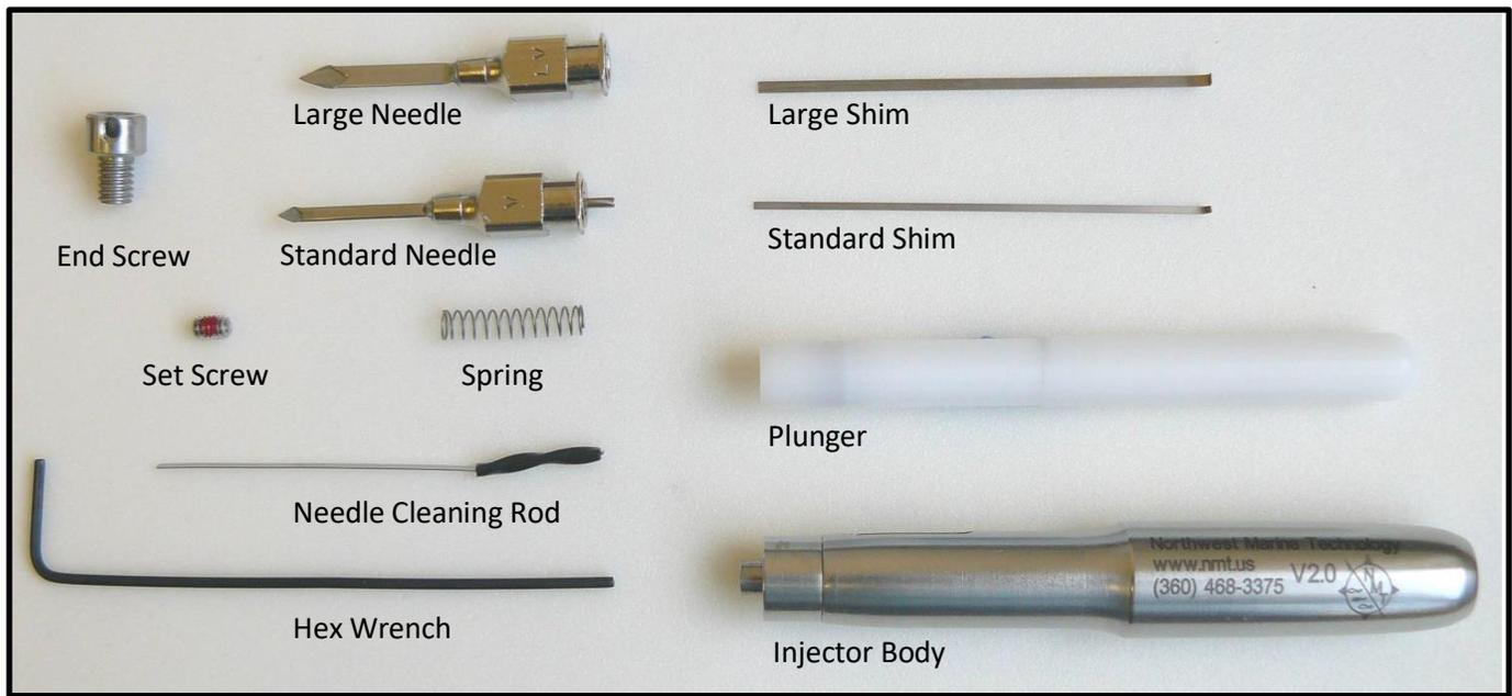
1. Insert the shim into the end screw with the bent end of the shim at the bottom of the screw.
