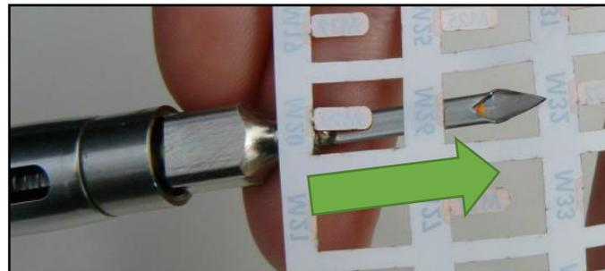
5. The tag is ready to be injected. Detached tags can be difficult to load, particularly when they are wet. We recommend holding one end of the tag with tweezers and inserting it into the needle.
