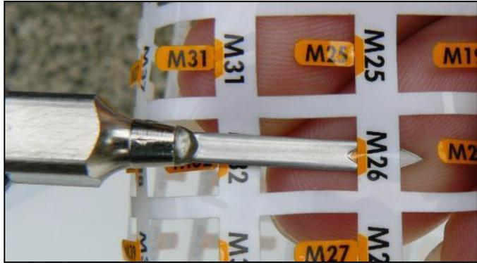
3. Keeping the tag pushed into the needle, fold the tag sheet back until it is flush with the needle, and the tag sheet is upside down. This bends the joint between the tag and the tag sheet.
