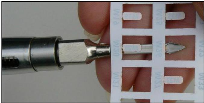
4. Push the injector forward to cut the tag. Do not twist the injector to remove the tag. Twisting will distort the tag material at the joint with the sheet. The tag will not load completely into the injector, and will not lay flat after injection.
