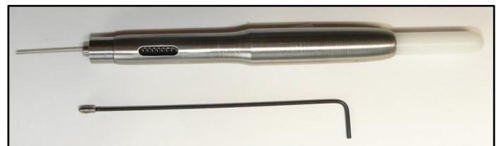
5. Rotate the plunger until the hole in the end screw aligns with the cutout in the side of the injector.
