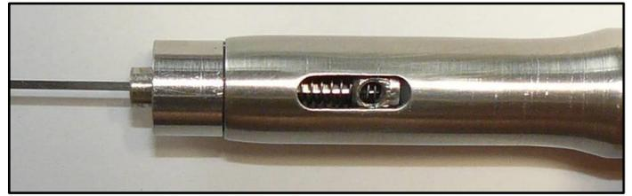
6. Insert the set screw and tighten it until it is flush with the outside of the injector body.
