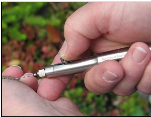
Figure 2: A Single Shot Injector is used to inject precut Sequential Coded Wire Tags.
