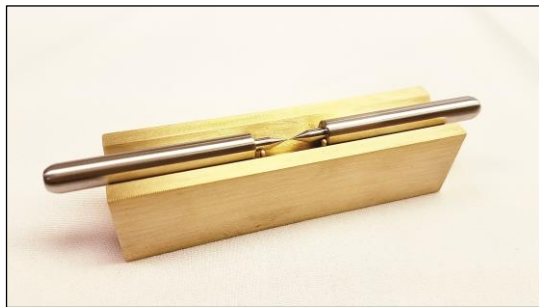
Figure 4: Tag Reading Jig with Pencil. The CWT is held between the tips of two pencils so that the tag can be rotated under a microscope.
