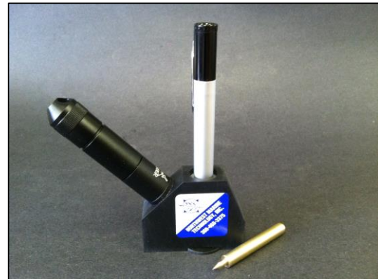
Figure 3: The Magniviewer is a portable, battery-operated device used to magnify and view CWT. Individual tags can be held with the brass pencil and viewed in the Magniviewer, or a strand of wire can be inserted into it. The Magniviewer operates on AA batteries and can be used anywhere.
