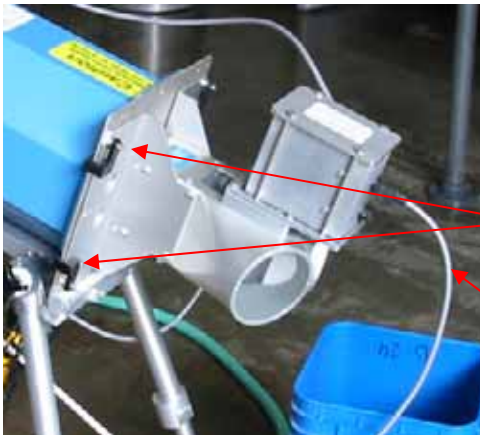
Figure 1- 18b: Gate brackets and gate attachment to detector.
