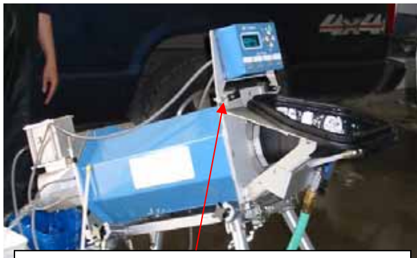
Control box with bracket attached to front of detector with wing nuts.
