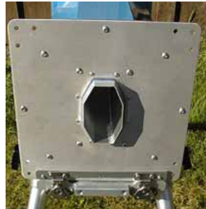
Front of detector resting in slot on legs; latches tightened
