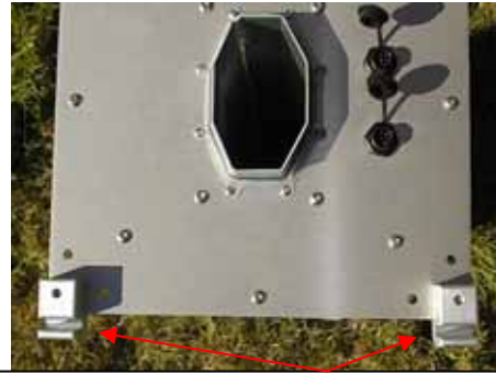
Rear end of detector showing alignment blocks that fit over pins on legs
