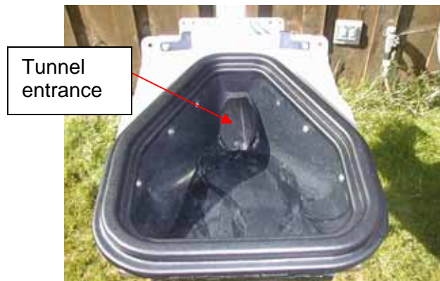
Figure 1- 7: Fish funnel attached to front panel of T4.
