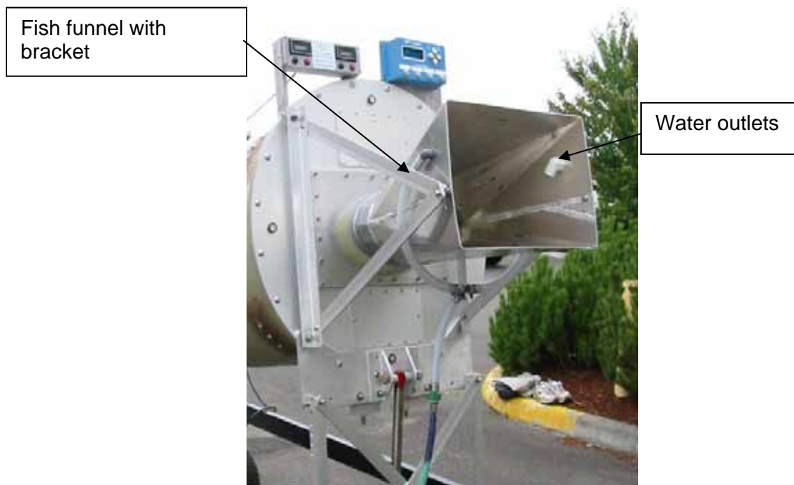
Figure 1- 6: Fish Funnel attached to front of T13 detector
