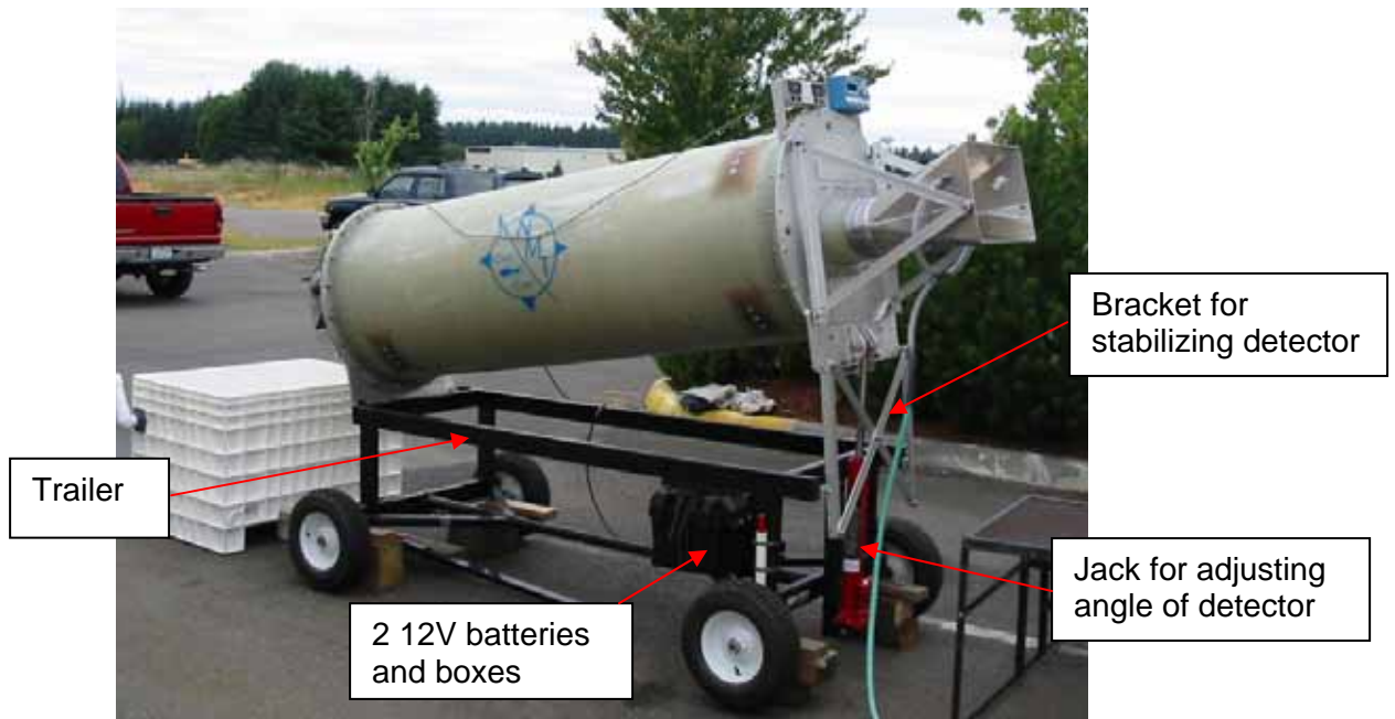
Figure 1- 7a: T13 detector with Diverter Gate and funnel on trailer
