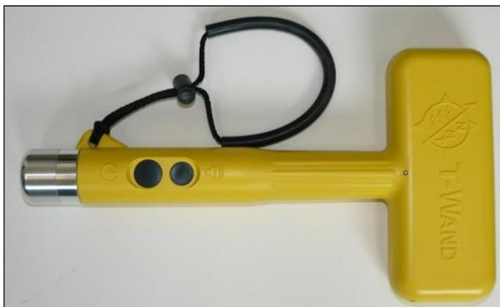
Half length tags have a detection range of about 2.5 cm, so their use should be limited to smaller species in which the depth of the tag could not exceed the range of the Wand. In body tagging, the tags are placed in different locations and their presence or absence is used to designate a particular batch. In these projects, the detection range of the T-Wand can be exploited to separate the body tag locations at recovery.
