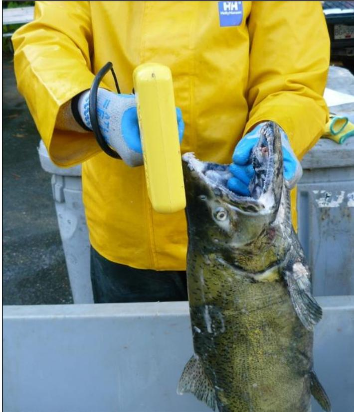
NMT's T-Wand is a rugged Coded Wire Tag (CWT) detector for field use. It is fully waterproof, floats, and is stable in a wide range of temperatures. It excels in field situations and in locations where transporting one of the larger detectors, and finding a stable base for it to operate on, can be difficult. The T-Wand can be used as a quality control device when tagging with a Handheld Multishot Tag Injector.
