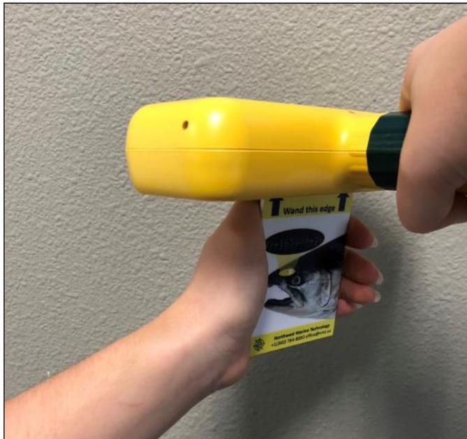
The CWT Detection standard is used to confirm that the T-Wand is functioning properly.
