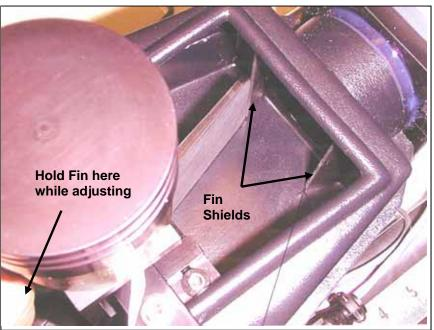
7. Move the Fin to the other side (left) and adjust the left bumper so the Fin's tip is flush with its respective Fin Shield (tag present).
