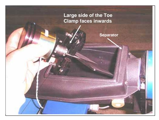
2. Slide the Toe clamp over the separator and line-up the Fin pin on the diverter assembly with the Fin bearing (rivet-shaped) in the separator section.
