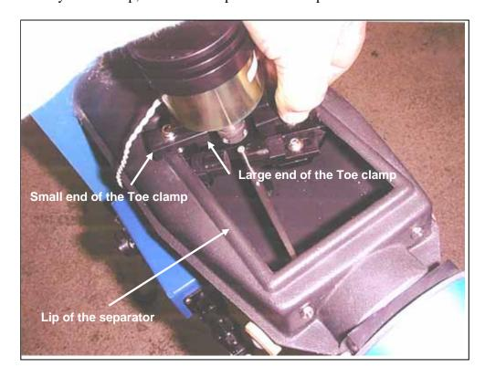
4. Tighten the two toe clamps down evenly – a little on one side followed by a little on the other side until the diverter gate assembly feels secure.
