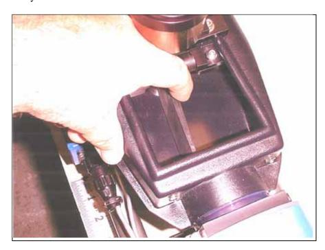
6. Set the right hand bumper stop so that the fin tip is flush with the Fin Shields. Hold the Fin in position while tightening the bumper. This will be the at rest position (no tag present).
