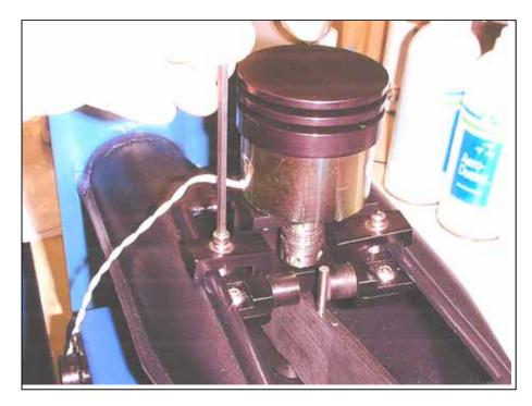
5. Make sure the fin moves freely. If the fin is not moving freely then readjust the position of the diverter assembly.
