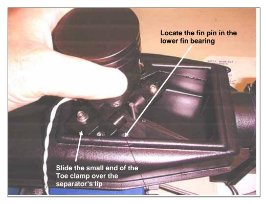
3. Rotate the other toe-clamp end into position. The diverter assembly should now have both of the toe-clamps over the plastic, and the mount under the plastic. Ensure that the "small" end of the toe clamp goes all the way over the lip, or riser in the plastic of the separator.
