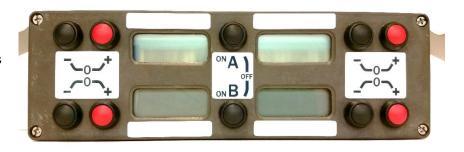
The left displays of each pair count fish exiting through the left door of the Gate. The right-hand display of each pair counts exits from the right door. If your fish are exiting to the side opposite of the display, switch the probes in the Gate doors. Each display has a pair of buttons labelled + and – that may be used
