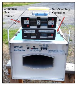
the cap on that second connector to keep it clean. The Combined Quad Counter can be stored with its door-switches attached, so long as the power is turned off. The gate switches cause a temporarily higher battery drain when activated. If a gate switch stays steadily active (door open or probe out of position) for 10 minutes, power will go off to save battery life.
