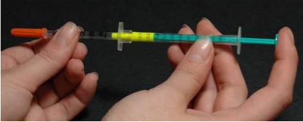
The tip of the 1 ml syringe fits tightly into the opening of the 0.3 cc injection syringe. Fill the injection syringe about 1/3 full. If you fill the syringe more than this, it becomes difficult to push out the elastomer and may result in a broken plunger.
