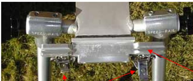
Front of legs. Slot for holding front end plate of detector
