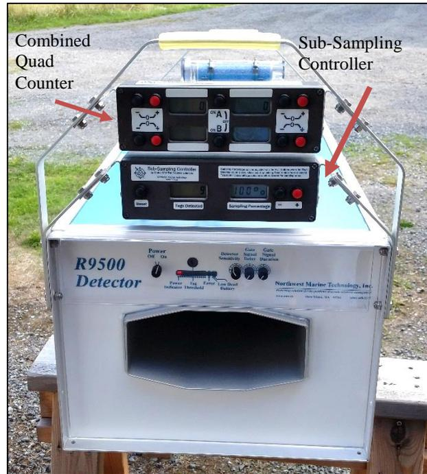
The front panel of the Sub-Sampling Controller is shown below. The + and – buttons adjust the sampling percentage, which is shown on the right display. The sampling percentage is the percentage of tagged fish that will be diverted. The left display counts all tag detections, including those fish that are detected as tagged but not diverted. The Reset button clears the counter when pressed and held for at least 1 second.
