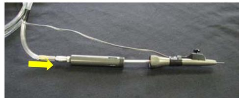
8. Hold the syringe housing and screw the cylinder body to it. The air hose connection fitting will rotate so the air hose will not tangle.
