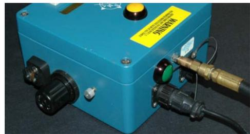
2. Disconnect the handpiece air hose from the control box.
